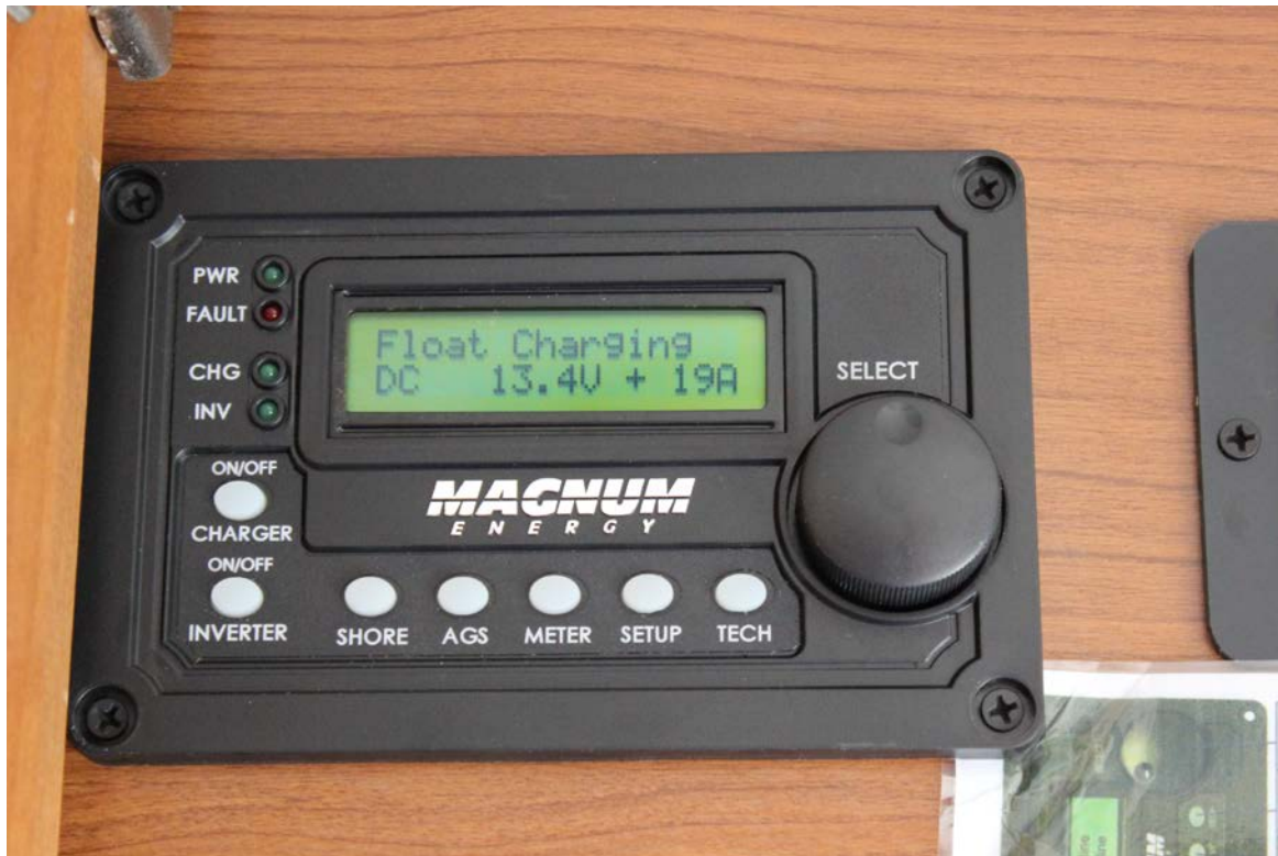
Figure 2-32: Energy management system
